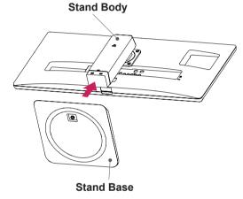
3 Using a coin, turn the screw clockwise to secure the **stand base**.
